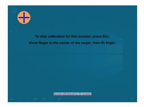
The Elo calibration tool is used to calibrate touch recognition on supported Elo touch screen monitors. After touching all 3 targets, the screen will show "Accept" and "Retry" buttons. The user can then test the calibration accuracy before selecting either "Accept" (saving calibration data) or "Retry" (re-doing the 3-point calibration).
