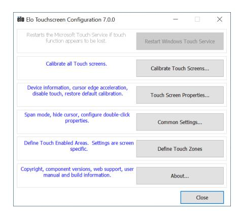
The following is a description of each of the buttons located in the Elo Touch Screen Configuration application:
