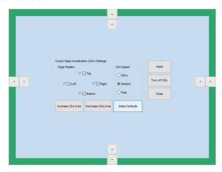
To enable CEA, click on the "Select Default" button and specify the desired parameters. The position of CEA may be manipulated for all edges at once by means of the "Increase/Decrease CEA Area" buttons, or individually by means of the arrows along each edge. Additionally, CEA for edges may be disabled by unchecking their respective box.
