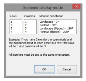
Enabling the "Spanned display mode" option followed by clicking the "Calibrate Touch Screens" button in the main EloConfig page will display a configuration window asking you to
