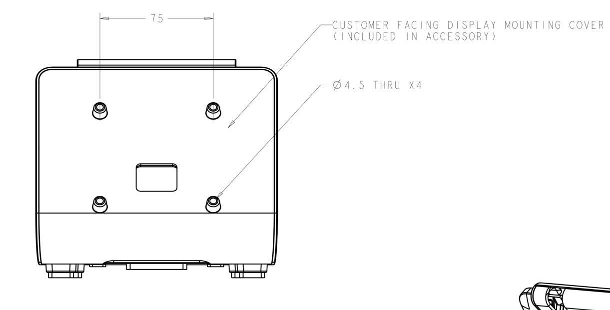
MOUNTING HOLES FOR CUSTOMER FACING DISPLAY X4—
